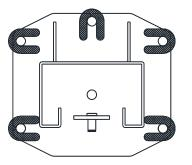
Fig. 3 – Column Shimming
