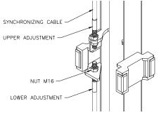
Fig. 6 – Synchronizing Cables
