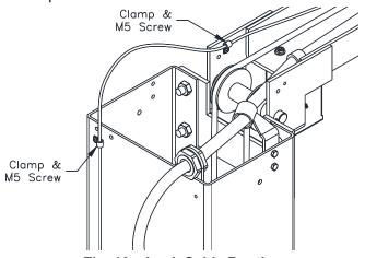
Fig. 10 – Lock Cable Routing
